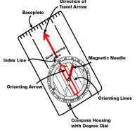
1. Line the direction of travel arrow up with the direction you would like to go or with the line of direction point A to B.
